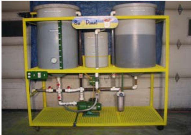
Len Aucoin, built a biodiesel production unit that supplies biodiesel fuel to operate his vehicles & heat his house & shop.
